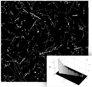
Illustration of single particle sensitivity of Timepix3 device. The tracks of different particles of radiation background (mostly muons and few protons) were recorded in 5 minutes on board of airplane. No noise (clean zero) is seen in dark regions. Inset shows the time profile along one muon track.
